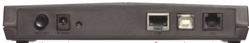
On/off switch Power jack for AC power adaptor RJ45 for 10/100 Ethernet LAN connection USB data port RJ11 for ADSL connection to telephone line
